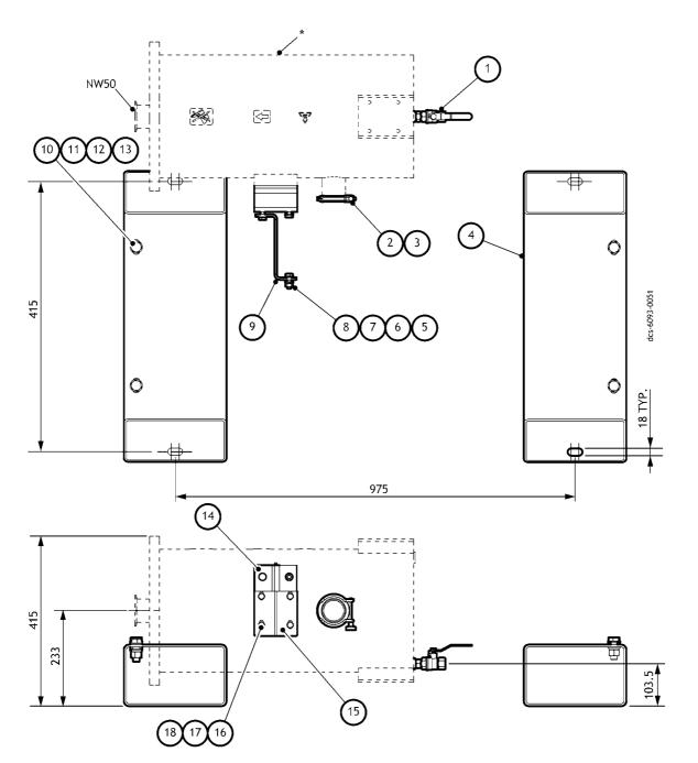
Figure 54 - M59838009 horizontal silencer mount - 150 ctr
