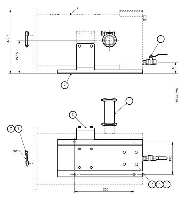
Figure 55 - M59808151 rear silencer horizontal mount - 150 ctr
